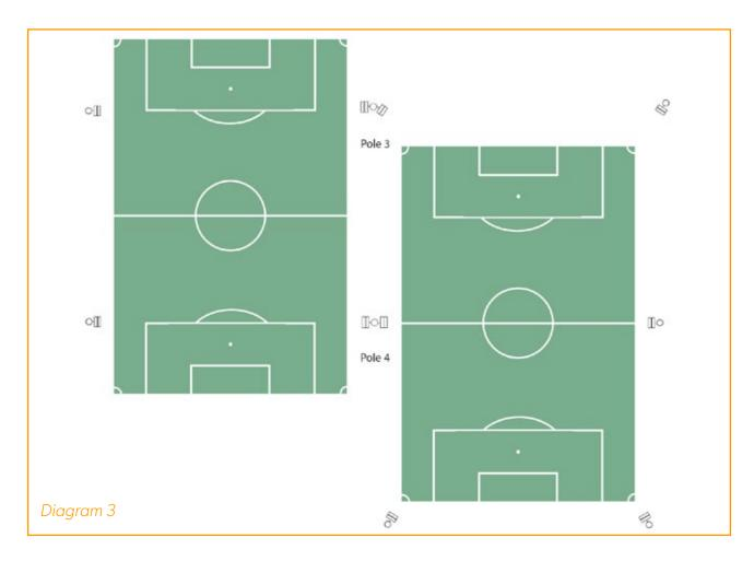
For floodlighting efficiency, offsetting of pitches is optimal where the offset is no more than 7m. This is because a four-pole side light design will generally look to position poles between 35-42m either side of the halfway line.
